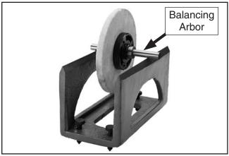
Figure 32. Wheel assembly on balancing base.
